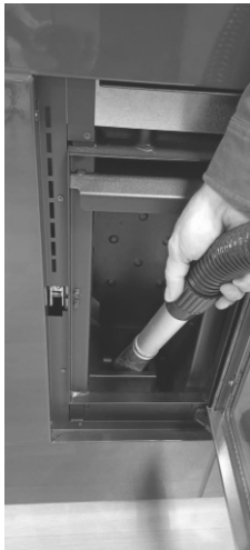
Fig. 35 - Burning pot box cleaning
