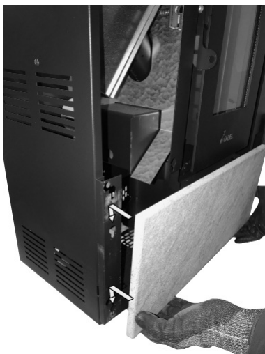
Fig. 30 - Hook the stone
