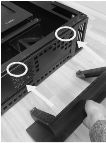
Fig. 53 - Position the stand
